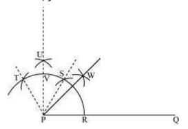
We have,  $\angle SPQ = \angle TPS = 60^{\circ}$ . In (iii) and (iv) steps of this construction, PU was drawn as the bisector of  $\angle TPS$ .
